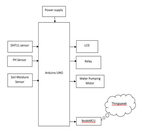
The proposed IoT-based precision farming system is designed to automate the monitoring and control of key environmental parameters essential for healthy crop growth, with a particular focus on optimizing water usage and improving overall farming efficiency. The system integrates hardware components such as Arduino UNO and NodeMCU (ESP8266) microcontrollers, which serve as the central units for data acquisition and communication.
